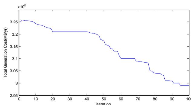
**Fig. 2.** Convergence characteristics of proposed GWO with 100 iterations (26 conventional + 2 wind units)
